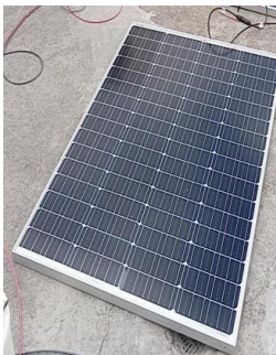
Figura 5. Panel monocristalino 160 W.
